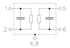
The recommended pin configuration usually offers best suppression of electrical crosstalk. The filter characteristics refer to this configuration.
